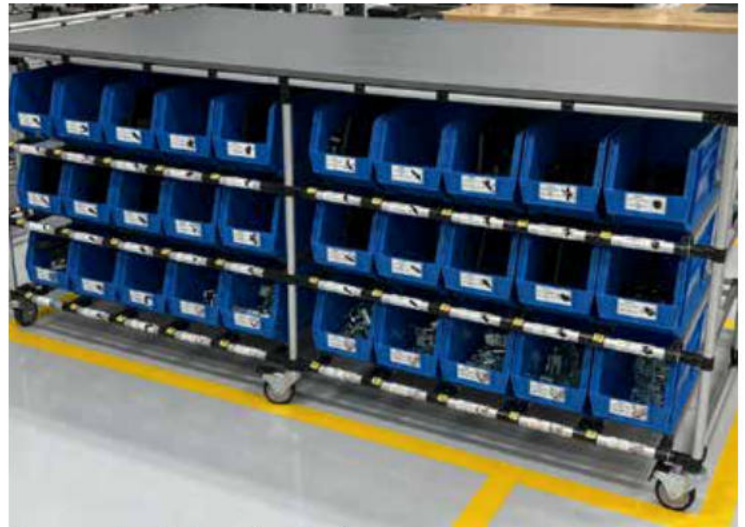
Supermarket Kanban Flow Rack
