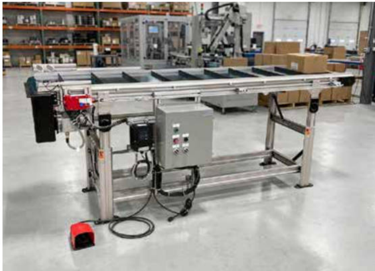
Single Strand Conveyor
