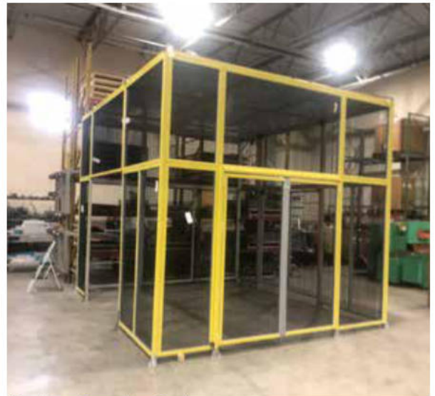
Machine Guarding Enclosure
