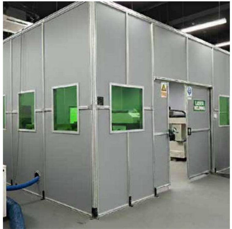
Industrial Laser Enclosure
